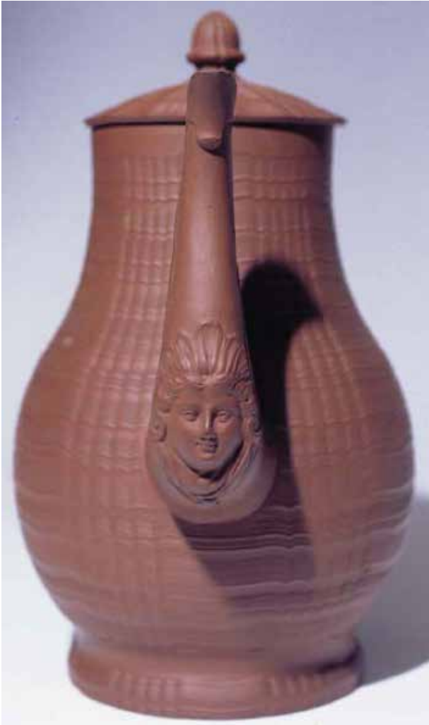
Plate 13. A wavy lined unglazed engine turned coffee pot with masked spout. The curved outline of the body shape when decorated using a wide cutter necessitates a change in the profile of each cutter used. A straight sided pot is a simple task in that the profile is constant.
