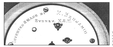
The backplate of the movement signed "Invented and made by M. Benjamin, Sydney, N.S.W." and the gold mounted jewelled pinion holes.
