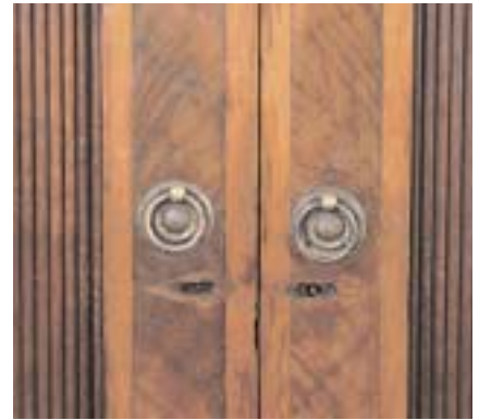
Plate 1c. Sliding tambour shutter fronts are difficult to make, being constructed from thin pieces of wood glued to a canvas backing. The brass handles are a later addition
